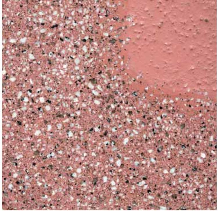
Granite based red Terrazite showing how the aggregate effect is exposed after diamond grinding of the applied surface (top right)
